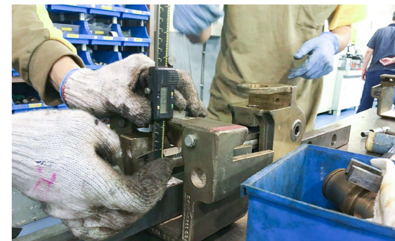
已打磨的制動鎖件正進行閉合衝程測試 The polished pawl locking housing is being tested for a closed stroke
